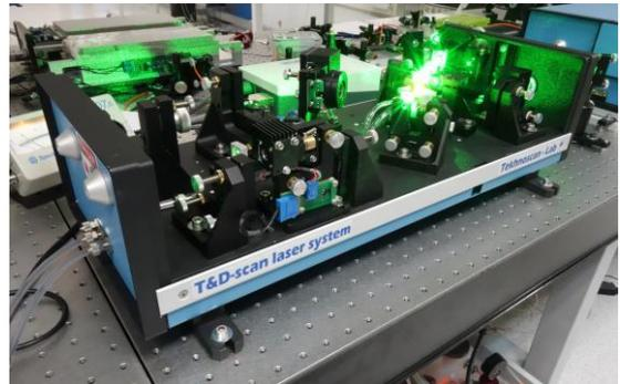
T&D-scan in Ti:Sa laser configuration
